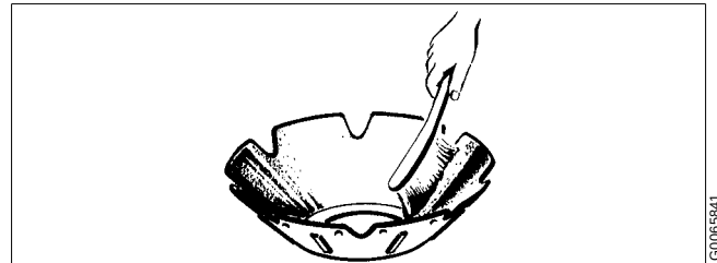
Clean the discs with a soft brush
