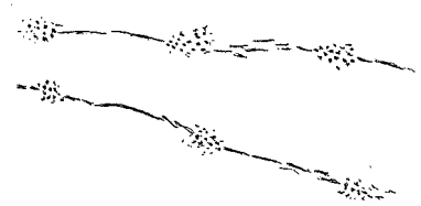
Example of chloride corrosion in stainless steel.
