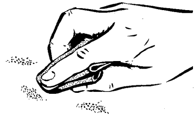
Polish corrosion marks to prevent further damage.
