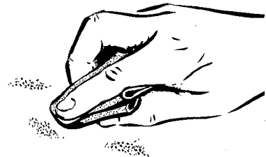
Polish corrosion marks to prevent further damage.
