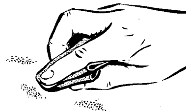
Polish corrosion marks to prevent further damage.
