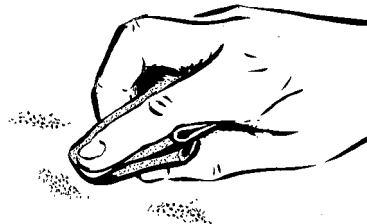
Polish corrosion marks to prevent further damage
