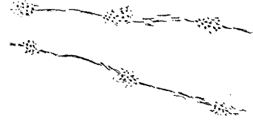
Example of chloride corrosion in stainless steel
