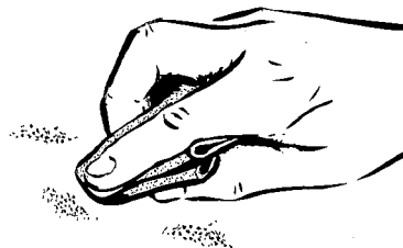
Polish corrosion marks to prevent further damage
