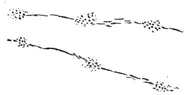
Example of chloride corrosion in stainless steel
